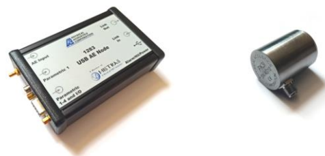
Fig. 1. AE monitoring system - flow-chart (top), Physical Acoustics data acquisition device (bottom left) and AE sensor (bottom right).
