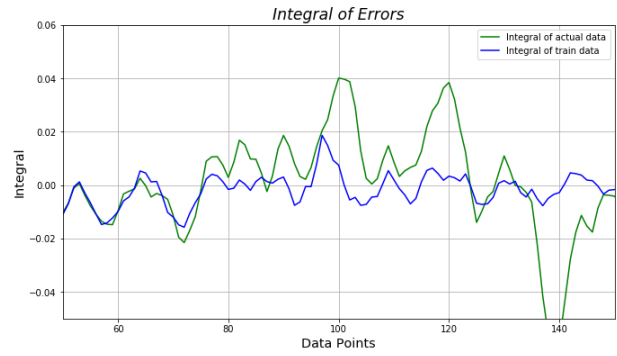
Figure 12 - Integrals of the error of the training data and the test data, for 6-point window.
