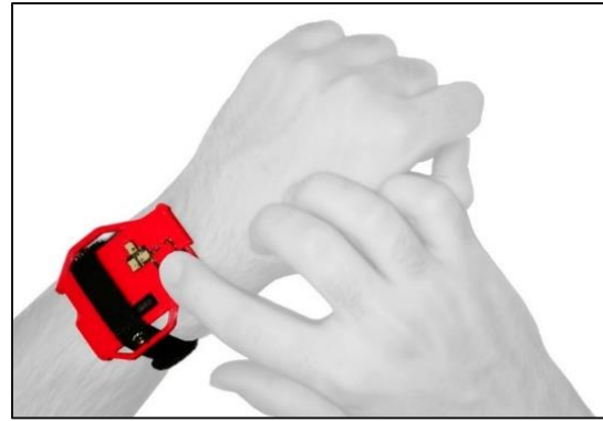
Figure 14. Board with enclosure and worn on the wrist
