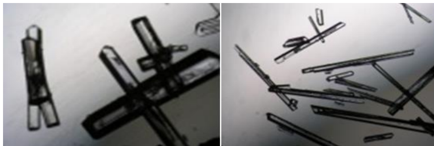
Figure 5. Micrographs of crystals of methyl tetra- O -acetyl- \beta -D-glucopyranuronate ( 1 ) grown from ethanol (left) in the absence of methyl tetra- O -acetyl- \alpha -D-glucopyranuronate ( 3 ) and (right) with 0.1:1 \alpha : \beta ratio.
