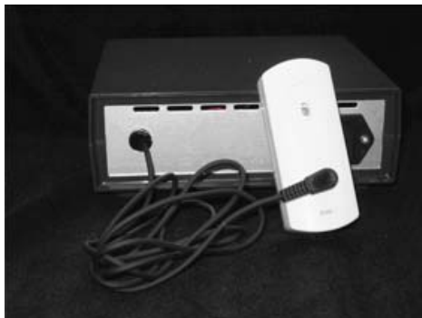
Wire at back of sound switch plugged into personal alarm
