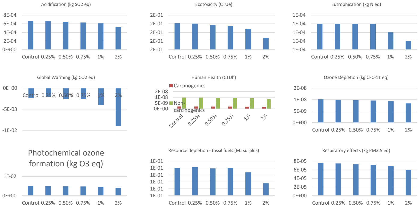
Figure S2-S7. Life cycle assessment impact metrics for the experiments at various PEG6000 concentrations.
