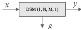
Fig. 12. Block diagram of the n -bit accumulator with an M -bit quantizer.
