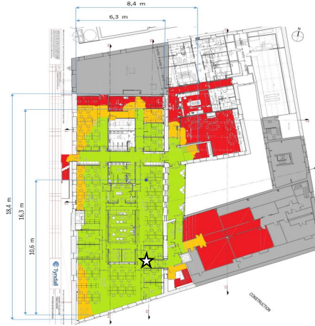
Figure 9. ZigBee 2.4GHz range test
