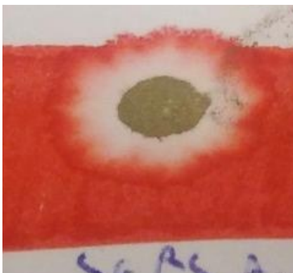
Figure S1. Photograph of commercial red felt tip line on paper with deposited Ag colloidal solution.
