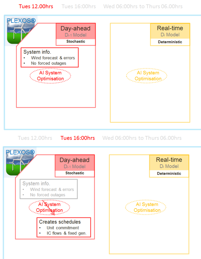
Figure 4.3: Flowcart representing the simulation steps of the DA and RT models' interleaved process
