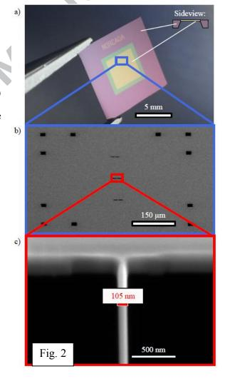
Superconductor (S-TI-S) junctions were consisted of Al evaporated via shadow mask on top of an Al-
